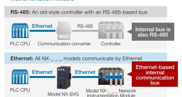
RS-485-based internal communication bus, data communications must wait for their turn. By contrast, the modules' Ethernet-based internal communication bus allows parallel communication, and its communication performance is overwhelmingly superior to that of conventional controllers.
