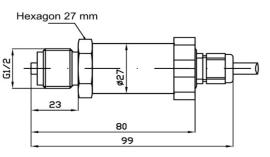
option, IP 67 oder IP 68 cable outlet with 2 meters securely connected PVC-cable,
