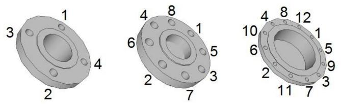
If the bolts are tightened too much during the installation or pipework components, deformation of the sealing surface may occur. In consequence, the torque values indicated in the table are used as a guidance for tightening the screws and bolts.
