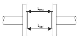
before the flow sensor is installed must not be greater than 0.5 mm.
