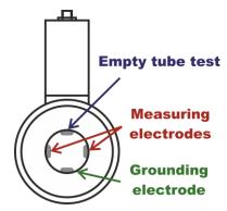
Installation in piping and placement of measuring electrodes in flow sensor
